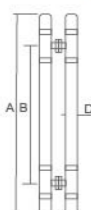
RL-DH024 Size(mm) A:600 B:400 D:φ38 A:800 B:500 D:φ38 Colour:Chrome plate /Stain nickel
